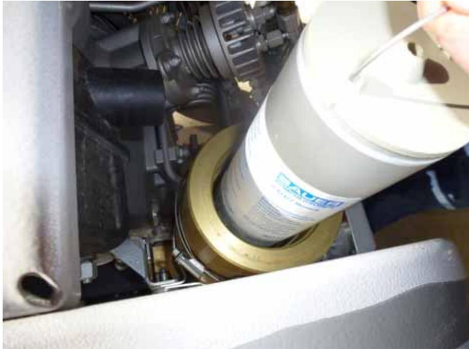
7. Open a new filter cartridge from the compressor box. Remove from the sealed bag. Remove both end caps. **NOTE – IF YOU DON'T REMOVE BOTH, THE FILTER IS VERY DIFFICULT TO REMOVE NEXT CHANGE**
