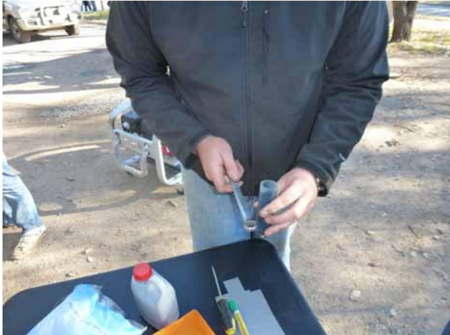
13. Fill to just below the spring line with 13x molecular sieve. Tap, cover with two cotton balls and tamp down.
