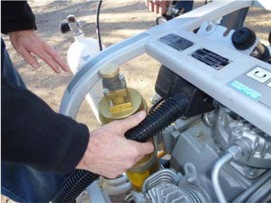
6. Check the engine oil (dipstick on engine). Top up if necessary.
