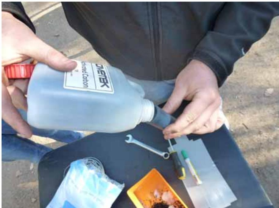
12. Tap the side gently for 10 seconds to get the carbon to settle. Place one cotton ball in the filter. Tamp down with the blunt instrument.
