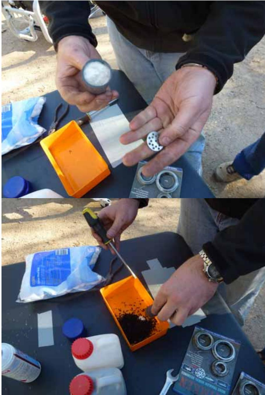
10. Make sure the cartridge is empty – you should see light through the hole. Place the disc in the cartridge, followed by two cotton balls.
