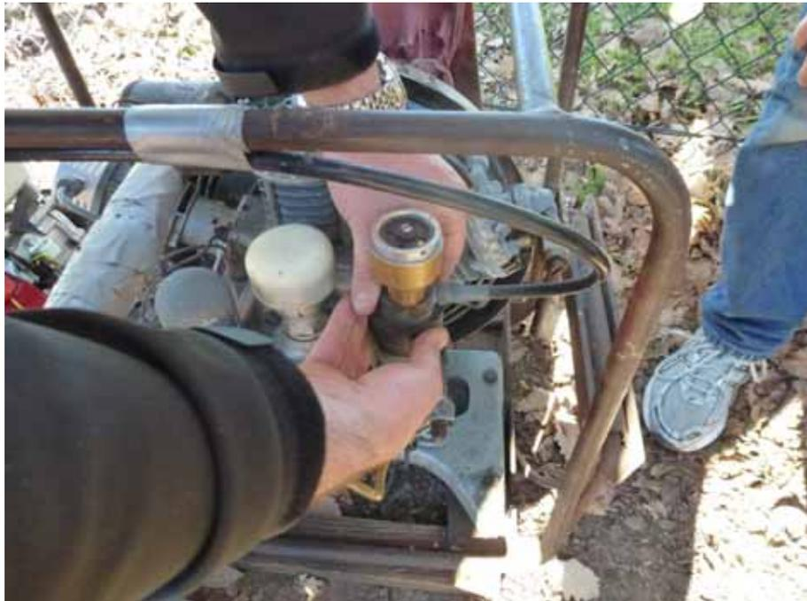
6. Unscrew the filter cartridge from the filter cap
