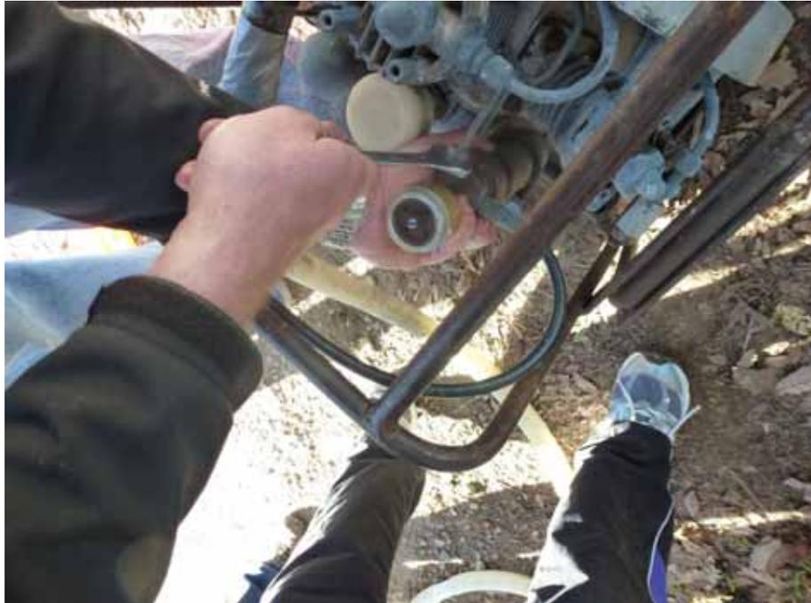
5. Unscrew the filter housing. This can be quite stiff. Note that it might seem to stop turning, until you apply some upwards pressure to the cap (use the gold coloured over pressure relief valve).
