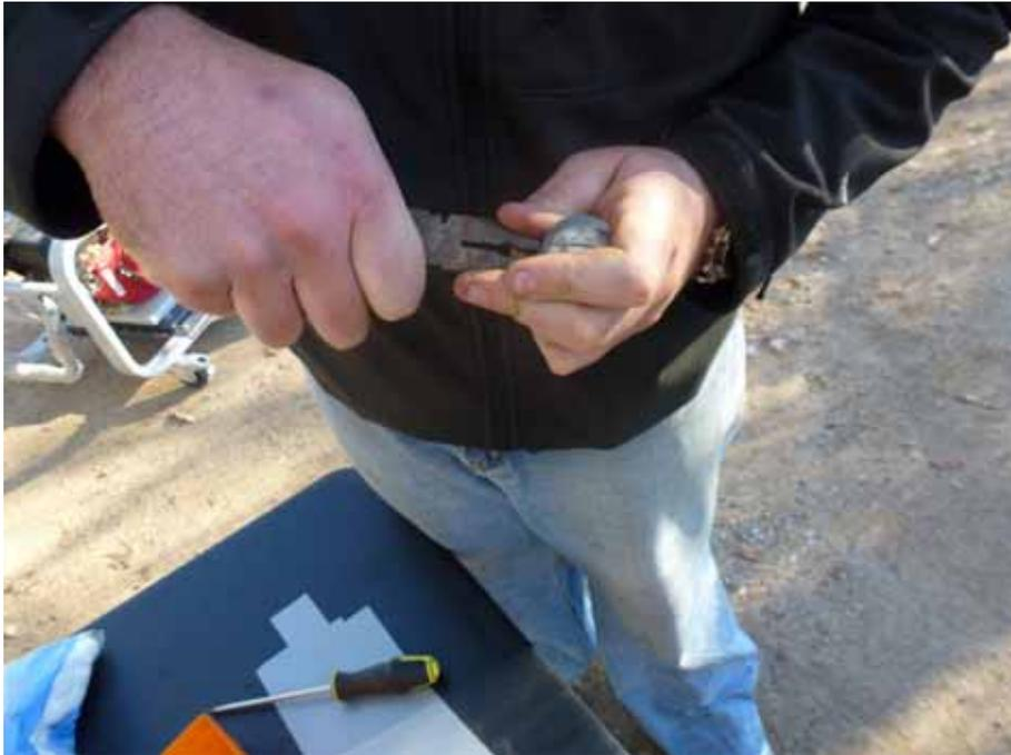
9. Empty the cartridge into a container. Keep the two perforated metal discs.
