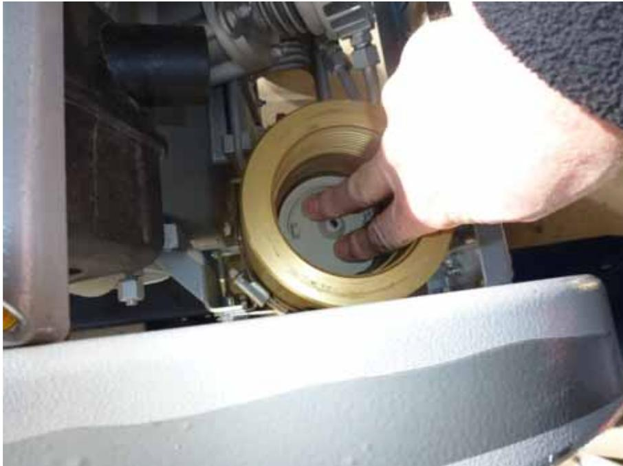
9. Check the o-rings on the filter cap for grit and debris. Clean if necessary. Screw the cap into the top of the filter. Tighten gently – only two fingers tight on the bar.
