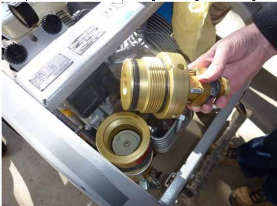
6. Remove the used cartridge using the metal handle. Using a permanent marker, write USED on the cartridge 3-4 times. This can now be disposed of. **DO NOT PUT IT BACK IN THE COMPRESSOR BOX**
