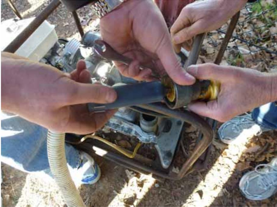
7. Take the filter cartridge to a clean place where you can work on it.
