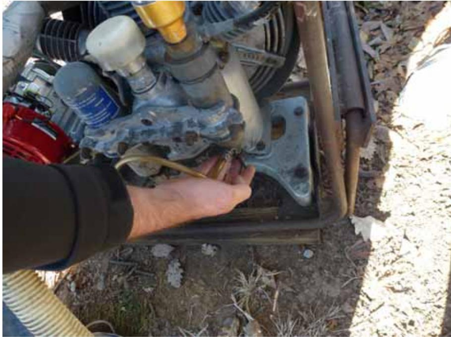
9. **IF THE COMPRESSOR DOES ANYTHING STRANGE, TURN IT OFF.** If the compressor runs out of fuel, let it cool down, refill (regular unleaded), and follow the startup procedure.
