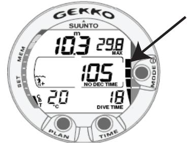
Fig. 3.11. Ascent Rate Indicator. Maximum allowed rate. Four segments
