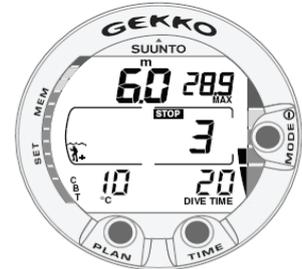
Fig. 3.9. A three minute Recommended Safety Stop.
