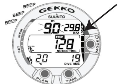
Fig. 3.12. Ascent Rate Indicator. Blinking depth reading, SLOW and four segments are shown together with an audible alarm: ascent rate is more than 10 m/min [33 ft/min]. This is a caution to slow down! STOP sign means that you are advised to make a Mandatory Safety Stop when you reach a depth of 6 m
