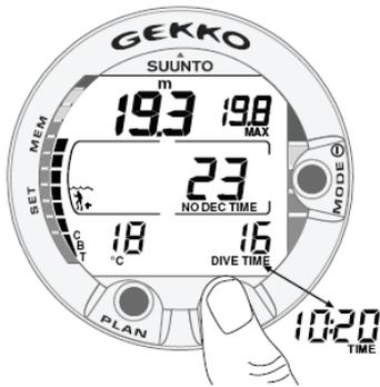
Fig. 3.7. Diving display. Present depth is 19.3 m [63 ft] and no-decompression stop time limit is 23 minutes in A0/P1 mode. Maximum depth during this dive was 19.8 m [65 ft], water temperature is 18°C, elapsed dive time is 16 minutes.
