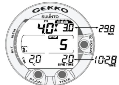
Fig. 3.13. A Mandatory Safety Stop. You are advised to make a 5 min Mandatory Safety Stop in the depth zone between 6 m and 3 m
